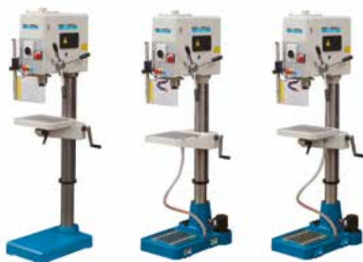
MG+R: Rotating table plate + coolant
