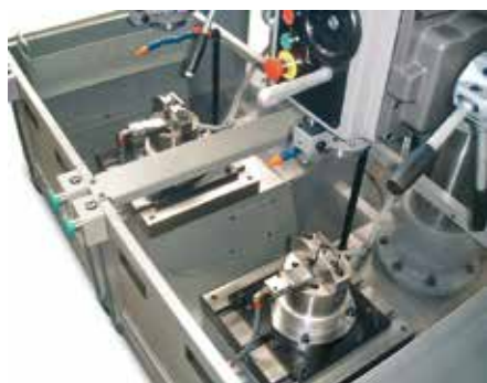
Hydraulic self-centering clamping tools for automation hinge.
