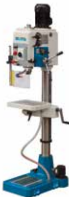
MG+R: Rotating table plate + coolant
