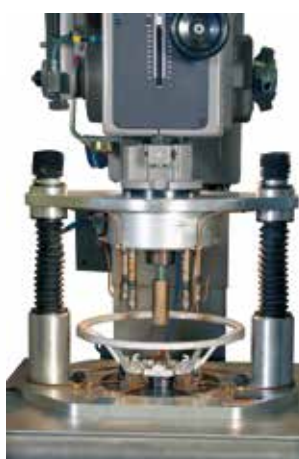
Multi-spindle headstock drilling detail of car handwheels.
